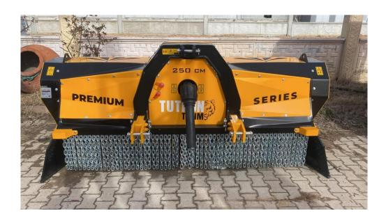
The Puma Stone Crushing Machine breaks stones on the field surface and up to a depth of 30 cm with the help of specially designed carbide diamond blades. The crushing process is carried out between 50 carbide diamond blades and Hardox plates. The interior of the machine is equipped with wear-resistant, replaceable Hardox plates.
